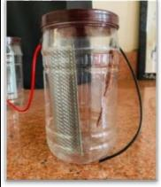
Fig. No.1. MicrobialFuel Cells
