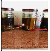
Fig. No.3. Microbial Fuel Cells withelectricity generated
